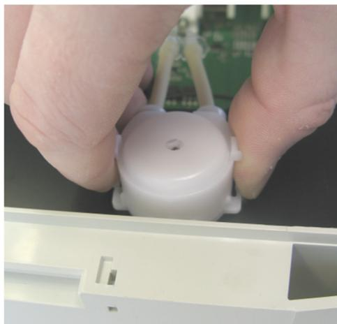
The pump unit has to rest on each side of the mounting plate and has to have snapped.
