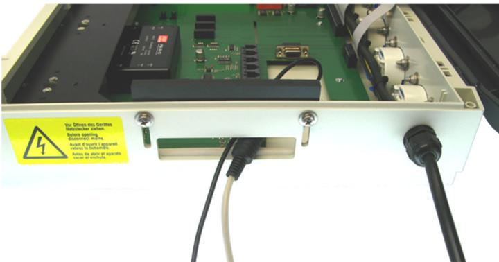
As soon as all cables are connected, the density mechanism has to be pushed together again. Place the cables here in a way that the sealing closes as densely as possible and tighten the screws well again.
