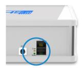
Located on the back panel of the *ION Director*® are another two LEDs that provide information about PAB connection status and PAB communication status.
