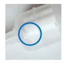
Make sure the tube is pushed all the way up to the filter housing. The filter connection sockets have a slightly larger diameter than the inside diameter of the sample water tube. This is purposely done to prevent the tube from getting disconnected.
