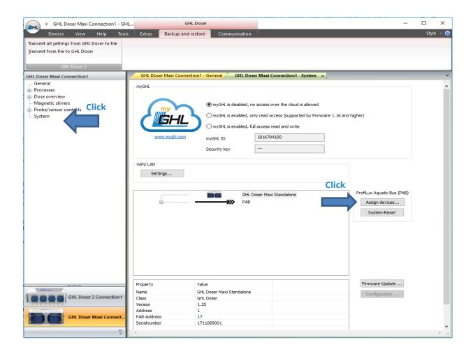
The Stand Alone Doser searches all devices connected to the PAB and then displays the serial number of the devices found. Then select the serial numbers of **all** devices that should be assigned to this *Stand Alone Doser* and confirm with *OK*.
