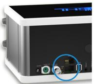
Located on the back panel of the *GHL Doser Maxi*, next to the connection of the temperature sensor are another two LEDs that provide information about PAB connection status and PAB communication status.
