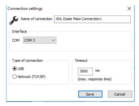
Now enter any connection name (For example, "GHL Doser Maxi") and set the previously determined port (*COM3*) via the selection window (<Auto>). Press "*Save*".
