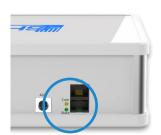
Located on the back panel of the *KH Director* are another two LEDs that provide information about PAB connection status and PAB communication status...
