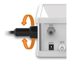
Tighten the screw connection as tightly as possible to prevent water from leaking out of the electrode, use an appropriate tool!
