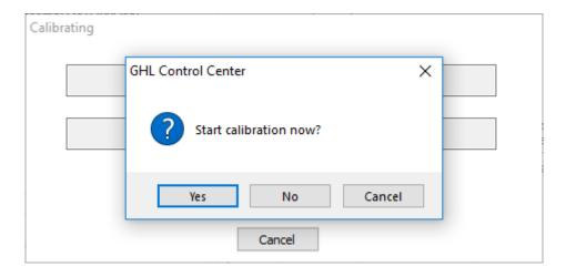
Prepare the **red** calibration fluid **pH 4**, immerse the electrode and start the calibration.
