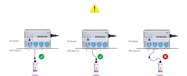
After connecting the tubes, the tube of the pump (here pump 2), which supplies the reagent liquid, must be vented.
