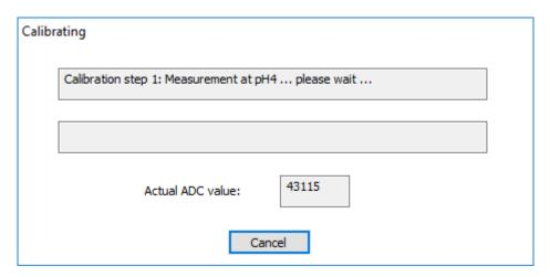
As soon as the calibration of the electrode to pH 4 has been completed, you will be asked to immerse the sensor in the **green** calibration liquid **pH 7**.
