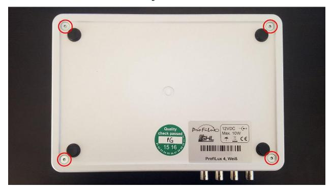
Using the 3/32 Allen Wrench, remove the 4 screws from the bottom of the ProfiLux 4.
