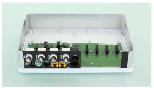
On the right, the empty slots for plugging in the modules are seen in the illustration above. On the left, you see the ex-works built-in Expansion Cards.
