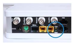
On the back of the *Expansion Box 2* are two status LEDs that provide information about the PAB communication.
