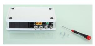
Turn the Expansion Box 2 upside down and carefully loosen the 4 Allen screws in the 4 corners of the housing bottom plate. Pull the screws out and reverse the housing together with the bottom plate again.
