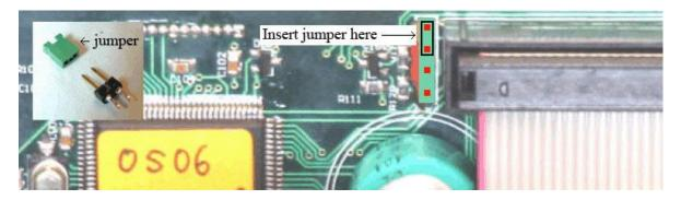
The jumper must be plugged such that the upper two contacts (pins 1 and 2) are short-closed.
