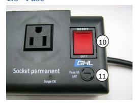
All sockets are connected to an illuminated switch (10) with circuit breaker function (UK-model without circuit breaker function). In case of an overload of the *Powerbar5.1-PAB*, this circuit breaker switches off. If the circuit breaker switch has been triggered, the switch can be switched on again after the overload has been eliminated. For the UK model, the overload protection is given by the fuse of the socket.
