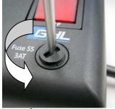
A defective fuse can be replaced by the user through a suitable replacement fuse with identical values (can be ordered as spare part). Other fuses are not permitted and lead to a loss of warranty. When changing the fuse, the powerbar has to be switched volt-free. You can replace the fuse by releasing the fuse element with a suited tool (e.g. slotted screw driver) with slight pressure inwards and a turn of ca. 45° counter-clockwise at the same time.
