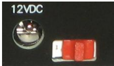
Figure 1 – Switch on the right: Device is switched on
