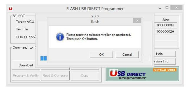
Now press and hold the reset button for at least 5 seconds, then release. Click "OK" on the above message and the download should start.
