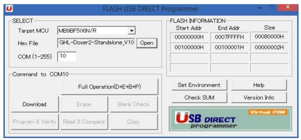
Load the firmware file by clicking "Open", then navigate to the firmware file and select it. You can find the firmware in the program directory of GHL Control Center. When you click "Open", select, "This PC", then:
