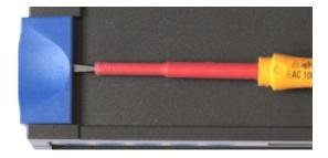
After all covering caps have been removed, the upper housing part can be removed. The housing is only stuck together, through releasing the 4 lugs, the housing can be opened. The easiest way to do this is to push a round item, ca. 5mm of diameter, from top into the housing locking. On the following picture a screwdriver is used for this.
