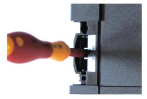
Tip: It will work especially easily if all 4 housing lockings (or at least 2 on each side) are released at the same time.
