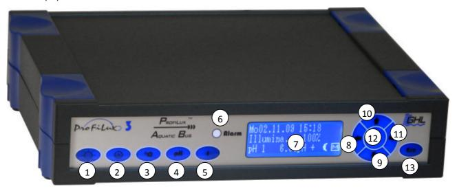
The keypad and displays of ProfiLux 3 (eX) aquarium computer:
