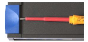
After all covering caps have been removed, the upper housing part can be removed. The housing is only stuck together, through releasing the 4 lugs, the housing can be opened. The easiest way to do this is to push a round item, ca. 5mm of diameter, from top into the housing locking. On the following picture a screwdriver has been used for this.
