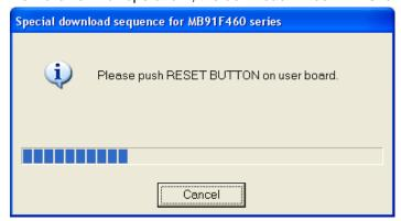
Press the reset key shortly and the download should start. If this is not the case, most likely the false interface has been selected under "Set Environment".
